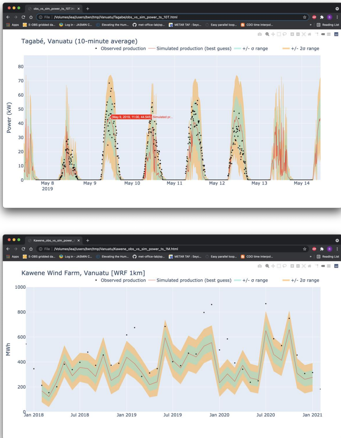
Figure 17: RE-SAT performance compared with observed production for the 80kW solar array installed at Tagabé (10-minute averages) and the 3.4MW Kawéné wind farm (monthly mean energy production). The black dots represent the observed power produced, the red line is the simulated production by RE-SAT, the colour bands are a representation of the uncertainty (1 sigma or 2 sigma)
