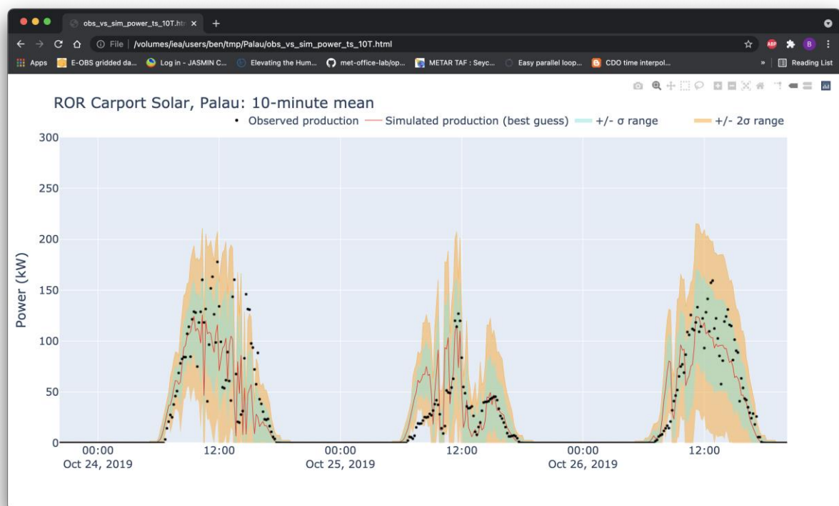
Figure 17: RE-SAT performance compared with observed production for the 236kW solar installation at Koror International Airport. The black dots represent the overserved power produced, the red line is the simulated production by RE-SAT, the colour bands are a representation of the uncertainty (1 sigma or 2 sigma)
