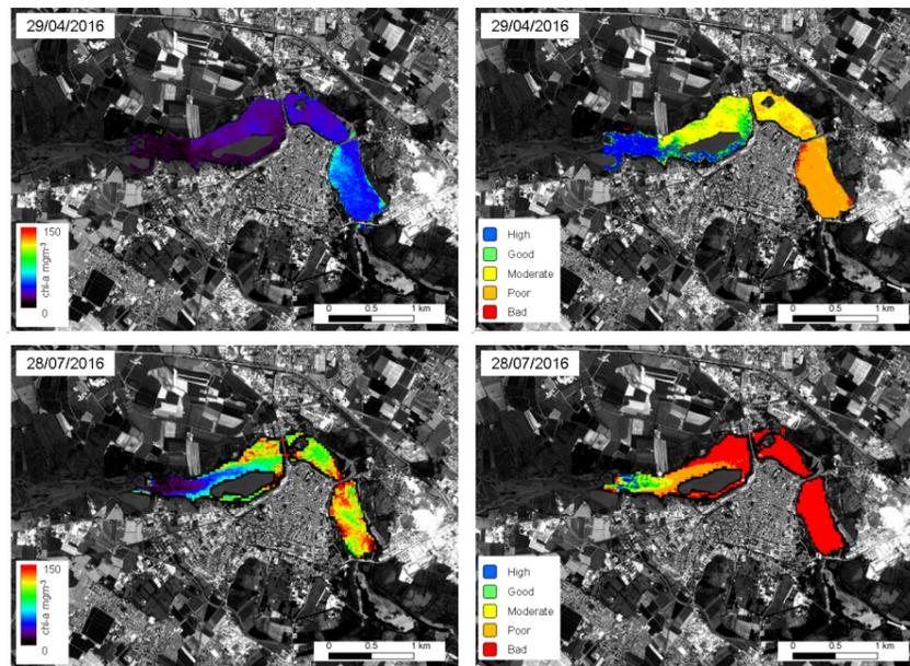
**Fig. 9** Sentinel-2 discerns chlorophyll-a concentration patterns over time, which are then converted into water quality according to the EC WFD supporting water managers of Mantua lakes (Italy). Credit: INFORM and BLASCO Projects
