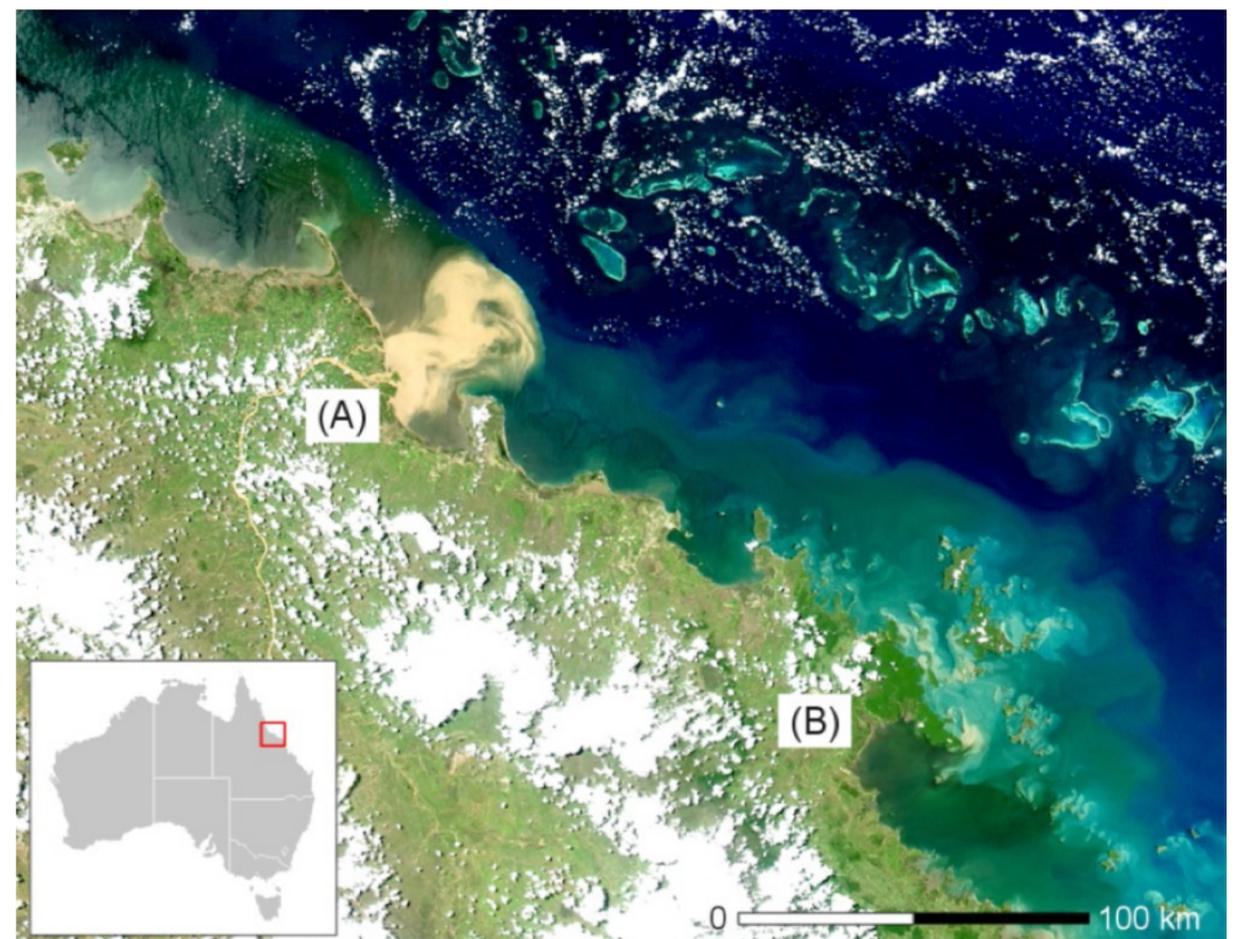
**Fig. 16** MODIS true-colour image illustrating the optical complexity of Great Barrier Reef coastal waters. Discharge of the Burdekin River (A) and the O'Connell and Proserpine Rivers (B). Credit: Schroeder et al. (2012, Marine Pollution Bulletin).
